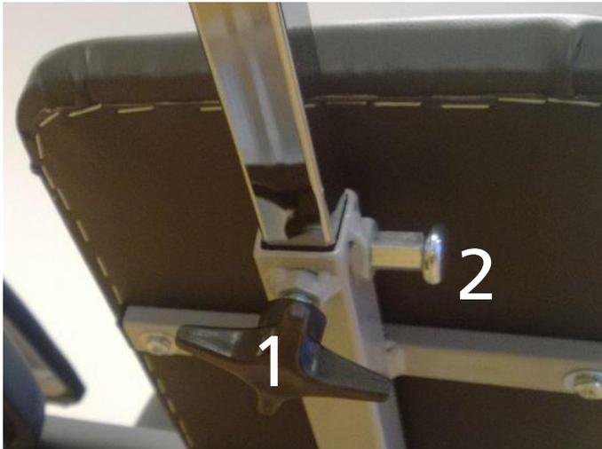
The heelrest position is manually and variably adjustable. To adjust, open the handle (1), pull out the heelrest to desired position and lock.
