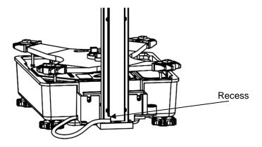
9. Remove the knobs [9] and mounting plates from the wall fixture [8].
