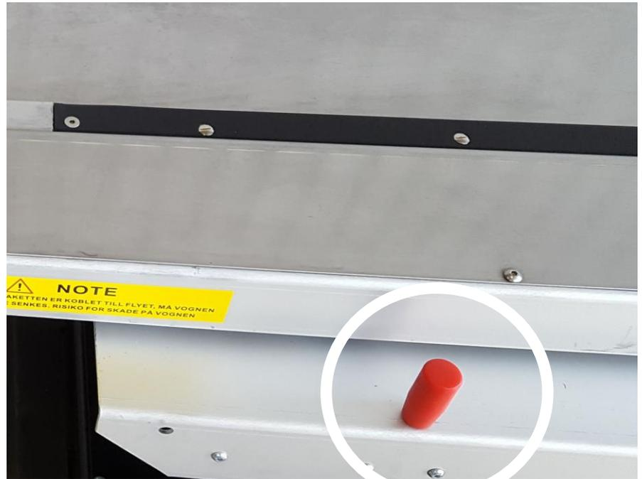
To release slide, pull out the fast-lock (cirkel) and pull out the slide.
