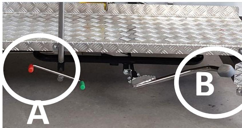
Lock the castors by pressing the red part of the pedal (A). Adjust the height by pressing B until it fits the airplane height. Release the slide and pull out. Make sure the slide height is slightly higher than the airplane attachment spot.
