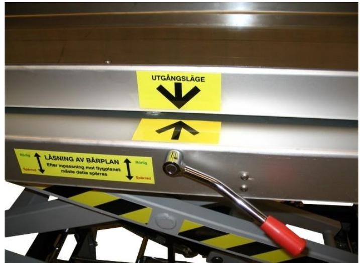
When the patient is moved from the airplane to the trolley, the slide should be pushed-in until locked by the fast-lock.
